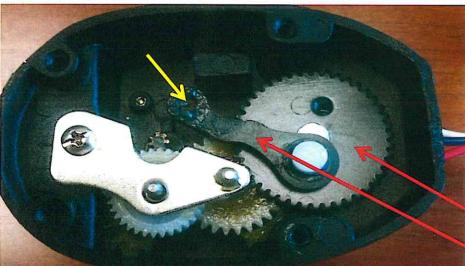
When the screws are removed, lift the silver plate up out of the motor can. As the top is lifted off, the pin on the motor crank will disengage from the hole in the link (where the yellow arrow is pointing).
