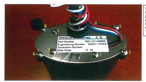
Once the pin on the crank is positioned into the link, push the motor plate flush against the motor can, and re-tighten the screws, in number order.
